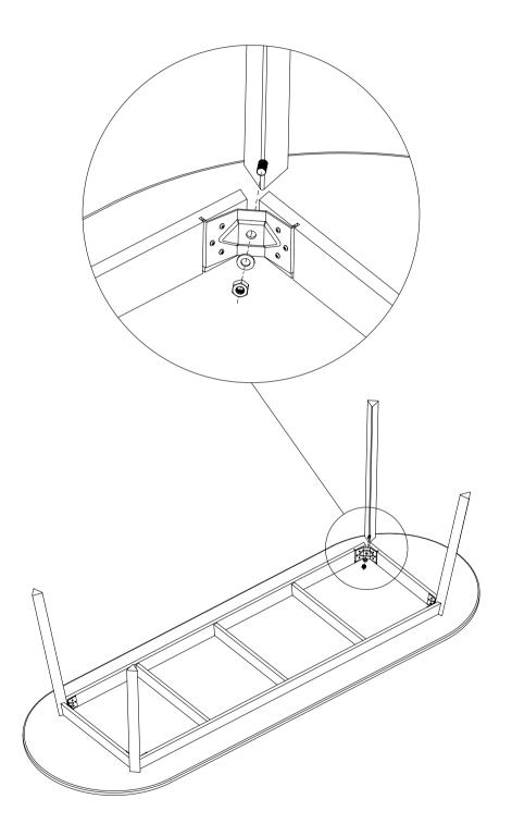
Use the E part to tighten the D part. Repeat the same procedure for all four legs.
