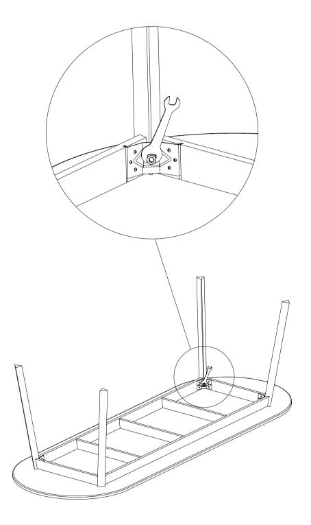
Turn the table over and make sure all bolts are completely tightened. (2 persons recommended).
